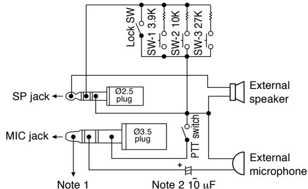
**Note 1:** Voltage is developed across the  $100\ \Omega$  resistor in the 3.5 V line in the transceiver. When 2 mA flows, approximately 3.3 V is developed.
